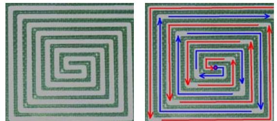
Not one spiral, but two! Follow red arrows to the center and return via blue to see signal spun inward and outward concurrently, as found on the KRT dual-spin coil antenna.
